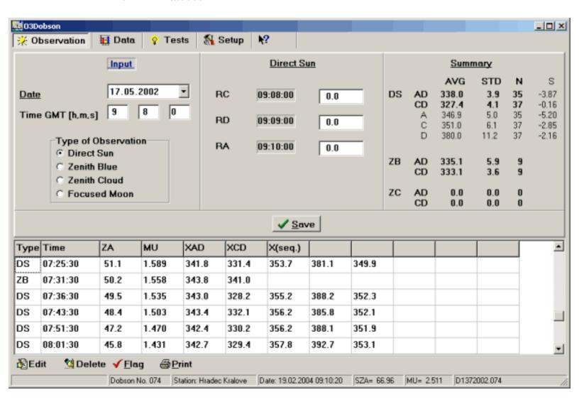
In the grid there are final results of each observation of the day - type of observation, time of XAD, Solar zenith angle, air mass, total ozone XAD, XCD, and XC, XD, XA - for CDA sequence. Daily summary is calculated and AVG, STD, N, and ETC correction (when N > 4 and MU range > 1) are displayed.
