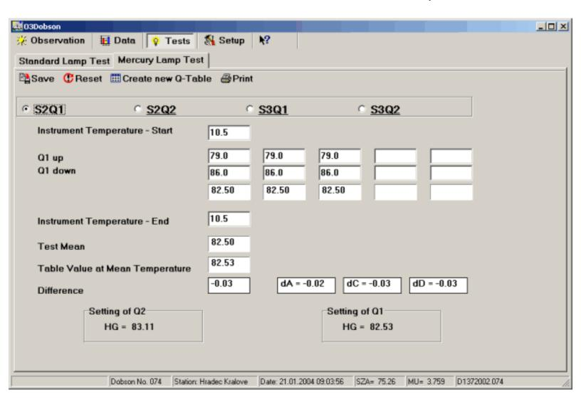
New Q-table is saved in a file and must be printed separately. The button "Create new Q-Table" change constants in Q-Table file automatically.
