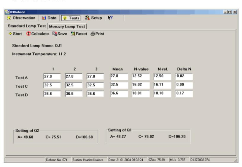
The correct setting of Q-levers is calculated based on the instrument temperature.
